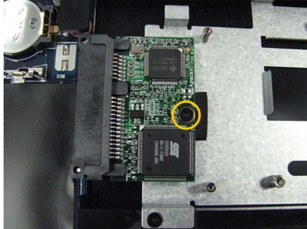
Figure 7 Removing the existing flash module
